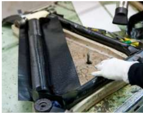
A Carbon fiber frame in production
